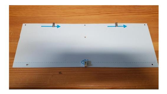
Use the 6 M3 lens headed screws to mount the bottom panel:
