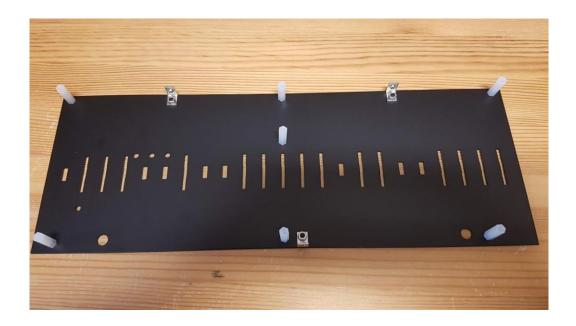
Next step is to fix the PCB using the 6 spacers with inner and outer thread
