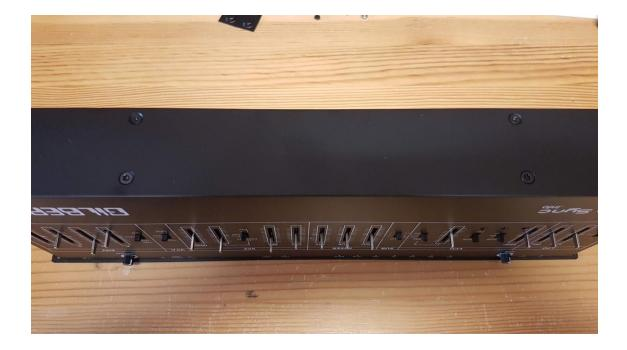
Now you can take the side panels and use the 8 tapping screws to fix them and the case assembly is nearly done. Last step would be to attach the 4 rubber feet and the slider caps.
