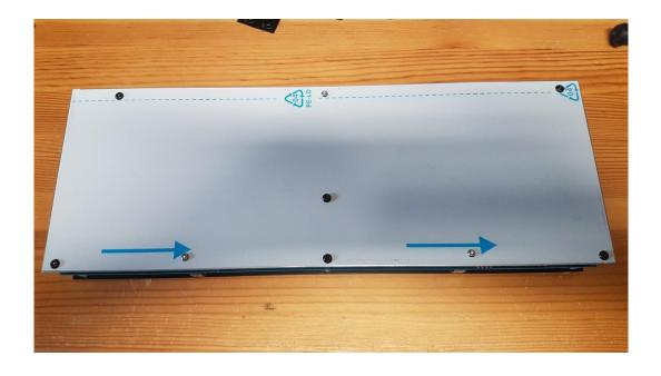
Now we are nearly at the end of the case assembly. We continue with the rear panel, the i/o sockets have to be installed flush and straight, otherwise the rear panel won't fit.
